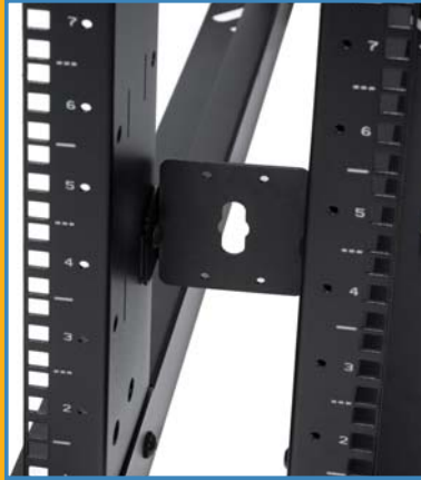
▲ Optional baying brackets tie individual Four-Post Racks together as well as provide mounting provisions for one power strip. Alternatively, Four-Post Racks can be bayed directly together for a reduced footprint.
