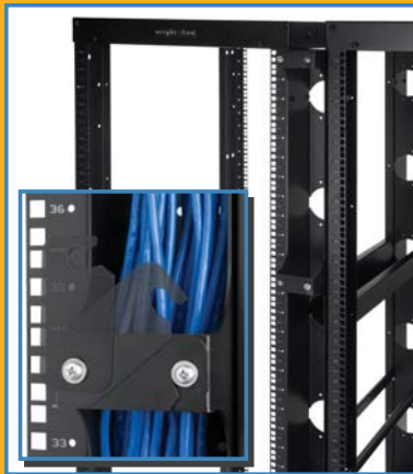
▲ The optional vertical cable management channel allows up to 288 CAT 5/6 cables in just one channel while maintaining a standard 24" baying scheme.
